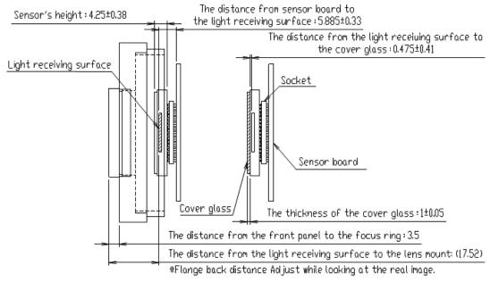
\*Cover glass's material:Labo-USQ (Can be changed to no glass model or AR coating cover)
