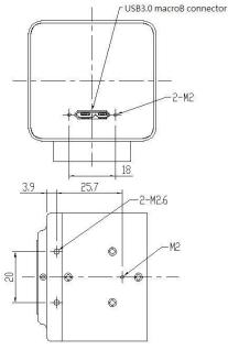
Drawing of the base without a tripod mount
